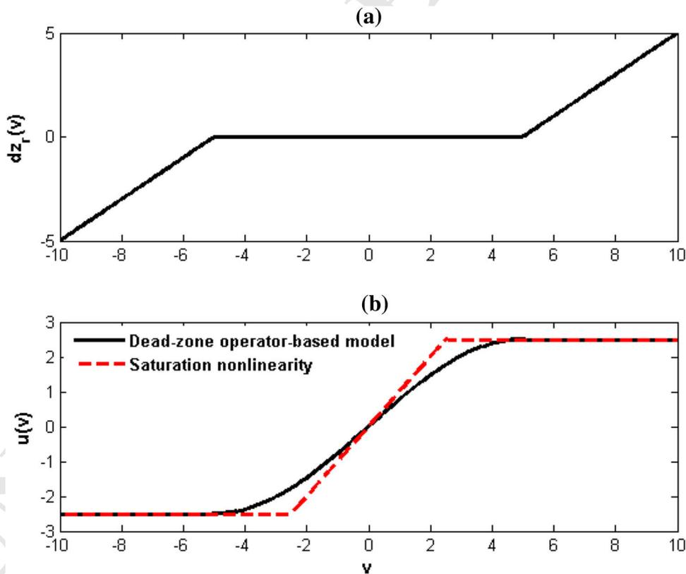
Fig. 1 a Dead-zone operator, b dead-zone operator-based model and saturation nonlinearity
