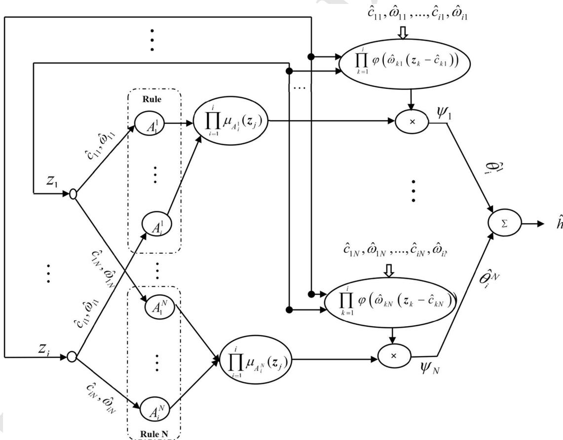
Fig. 2 Structure of the adaptive fuzzy wavelet network
